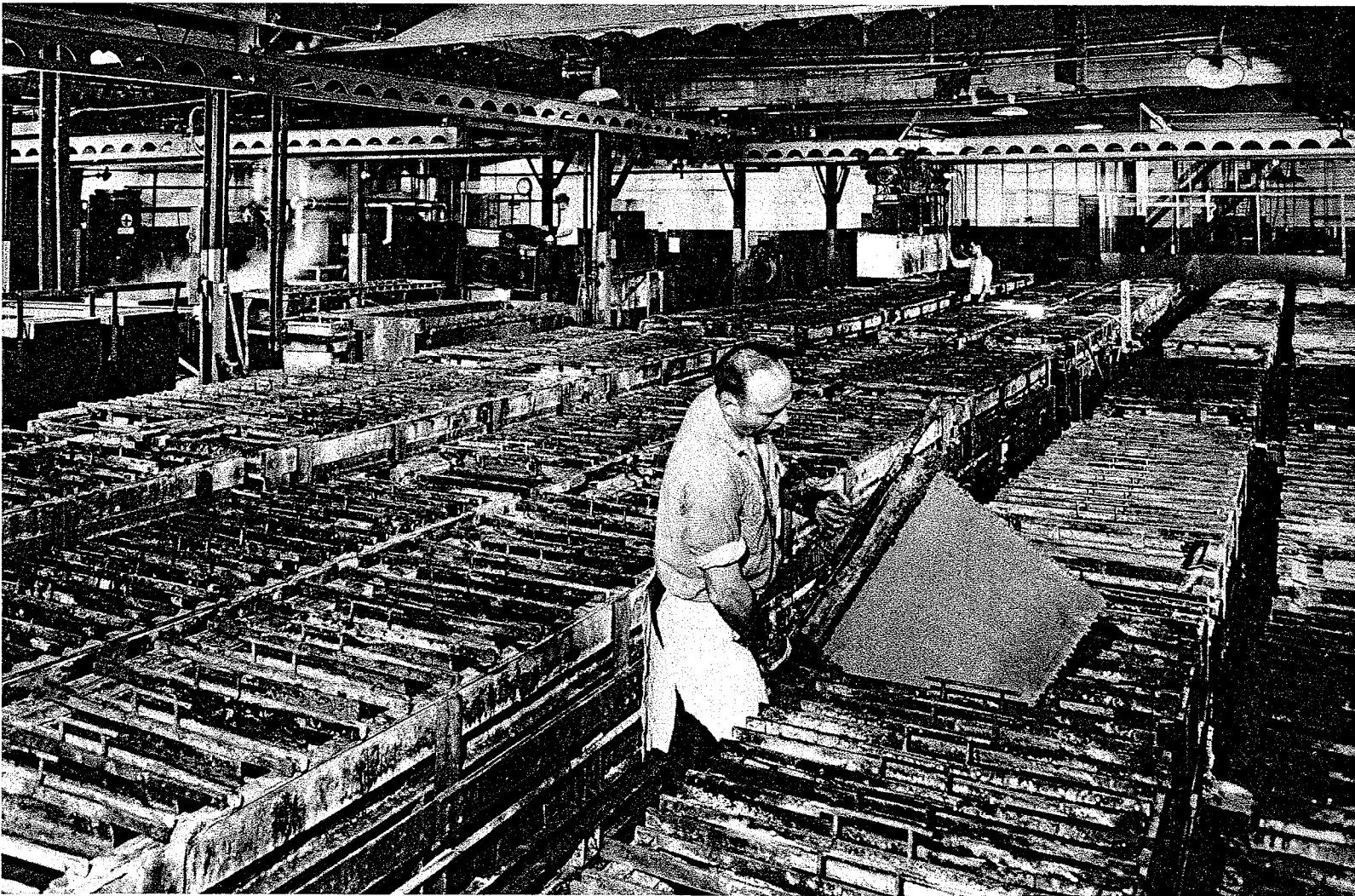
2—Electrolytic iron is produced in these electroplating cells.
